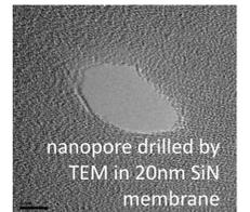
nanopore drilled by TEM in 20nm SiN membrane
