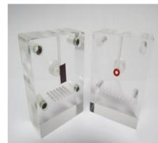
The chip is sealed by silicone o-rings between two reservoirs of a PMMA fluidic cell. Ag/AgCl electrodes are immersed into both reservoirs, filled with electrolyte, and connected to the instruments.
